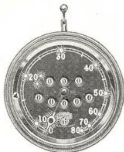
Figure 8. The Smith British Speedometer (Luminous Dials).
